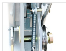
钢丝绳断裂保险机构。 Safety mechanism for protect quickly declined caused by wire rope breakage.
