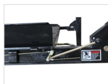
手动保险杆。 Manual safety bar for release.
