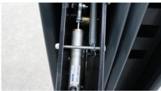
放气气缸 Air cylinder for air release
