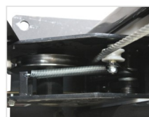
钢丝绳断裂保险机构。 Safety mechanism for protect quickly declined cause by wire rope breakage.
