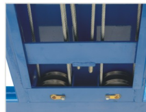
主跑道下方的钢丝绳和滑轮。 Wire rope and pulley under main runway.
